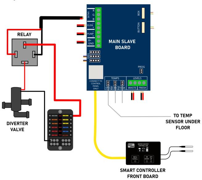
For simplicity, the above wiring diagram highlights the additional bits that you need to wire for the underfloor kit.
